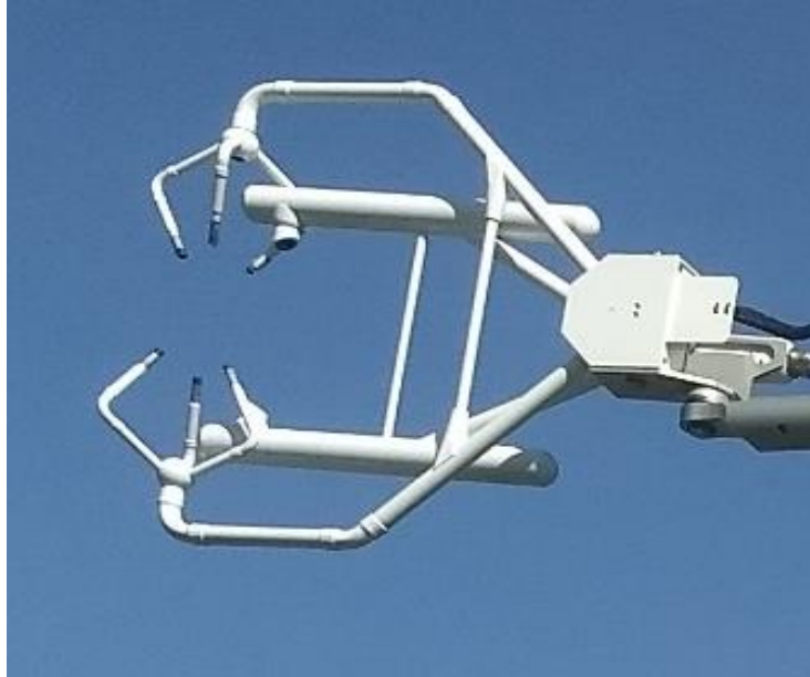
Fig. 3. 6 The Eddy covariance sensor installed at Nagani AWS station
