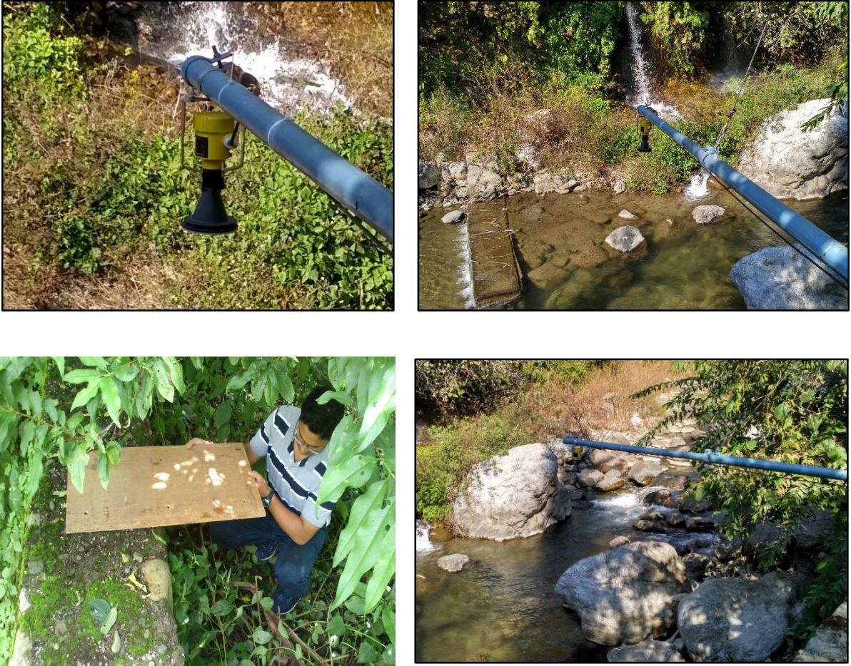
Fig. 3. 5 The digital water level recorder (DWLR) installed on the outlet of Henvai stream
